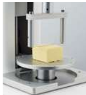
WIRE SHEAR FIXTURE (Ref. 130076)
