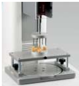
MULTIPLE PROBE FIXTURE (Ref. 130170)
