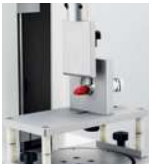
LIPSTICK CANTILEVER FIXTURE (Ref. 130147)
