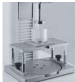
EXTRUSION FIXTURE (Ref. 100200)
