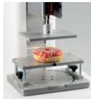
COMPRESSION TOP PLATE FIXTURE (Ref. 130153)
